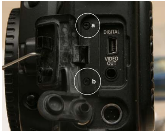
Figure 1. Removal of left cover (screws a, b)
