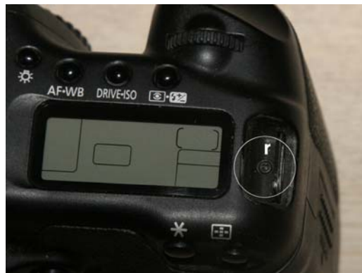
Figure 9. Removal of top cover (screw r)
