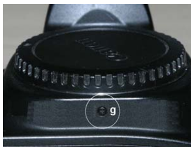
Figure 3. Removal of front cover (screw g)
