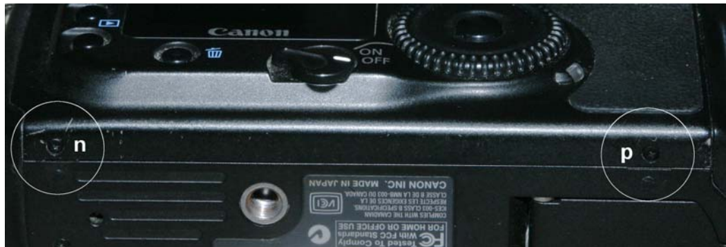
Figure 6. Removal of back cover (screws n, p)
